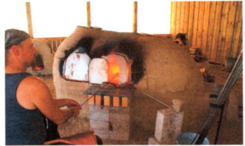
Abb. 5: Glas blasen direkt am Wannenofen GO-Borg-3. – Blowing glass directly in front of the tank furnace GO-Borg-3.
