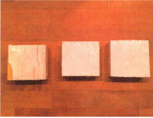
Abb. 1: Links: kein Harz, Mitte: 25%, rechts: 50% Harz-Zumischung. – Left: no resin, middle: 25%, right: 50% resin added.
