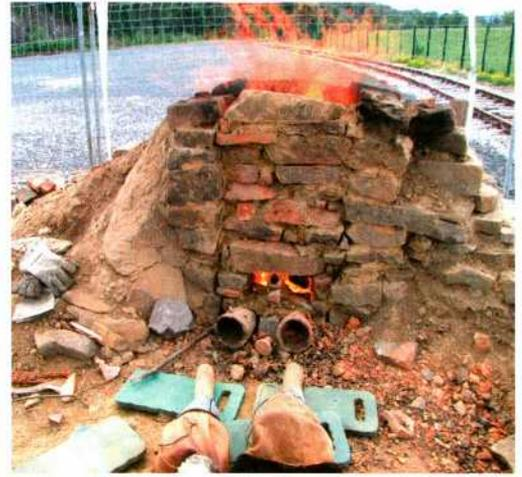
Fig. 5: Third furnace, built on the ground of the LWL-Industrie Museum Henrichshütte, Hattingen, Germany. Here two sets of tuyeres were used: one was attached to the bellows and was loosely set into a second tuyere that was entered into the furnace. This was done to keep the backdraft from the furnace from burning the inside of the bellows. The small clay pipe in the middle was used to measure the temperature. The area above the tuyeres was kept closed with clay and stone during the smelt.
