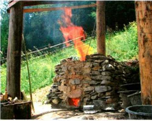
Fig. 3: First furnace, built near the mine "Arthurstöllen", Mitterberg Mining District, St. Johann in Pongau, Austria. Preheating the furnace with wood, without the use of bellows.
