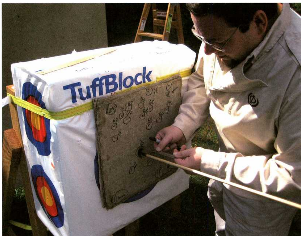
Fig. 5: Measuring penetration of arrow into test patch.
