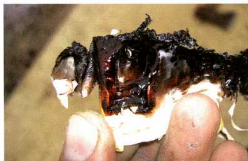
Fig. 4: After heating between 10 and 25 minutes, this method yielded small amounts of pitch.
