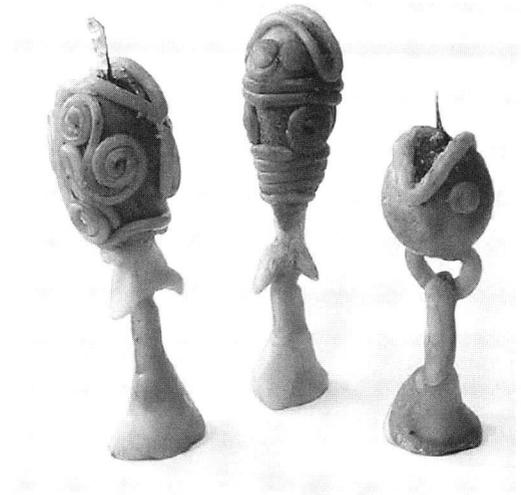
Fig. 6: Designs in wax with the casting channel.
