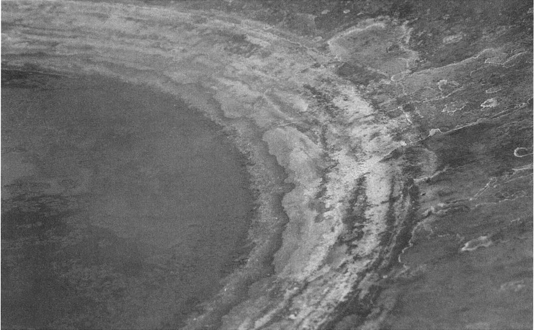
*Fig. 11: Crystallization of salt in the pan during the first Archeon experiment.*
