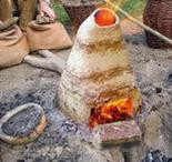
Copper ore together with charcoal had to be heated up to 1100° C in a shaft furnace constructed of clay. For the chemical reaction oxygen was needed, which was pumped into the furnace with bellows. The precious metallic copper emerged on the ground of the furnace.
